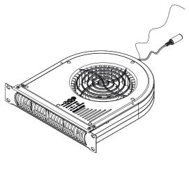
NOTE(S): FAN SPECIFICATIONS: AIRFLOW: 50 CFM [1.4 M3/MIN] CURRENT DRAW: 420mA @ 12 VDC SOUND LEVEL: 28 dBA @ 1 M STATIC PRESSURE: 0.31 IN H20 [77.22 Pa]
