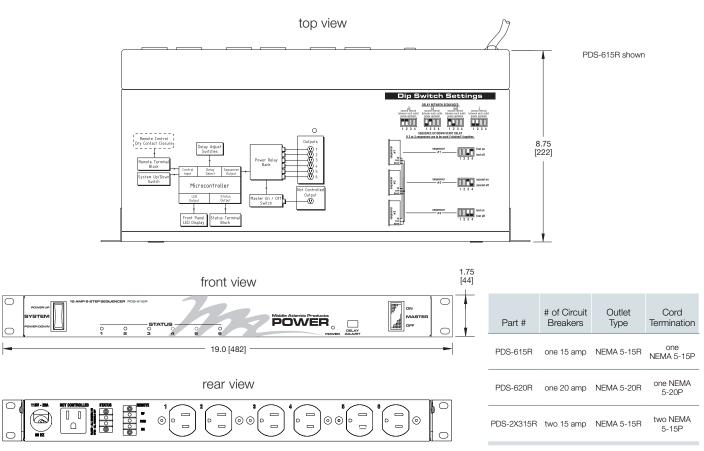
Maximum Derated Load (North America) for 15R Models: 12 Amps for 20R Models: 16 Amps
