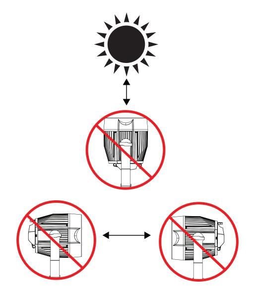
**NOTICE:** The maximum ambient operational temperature for this lighting fixture is *113° F (45° C)*. Do not place this lighting fixture in an environment where the temperatures exceed this value. This will allow the fixture to run at its best and help prolong the fixture life.
