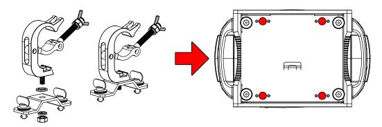
Tighten the quick-lock fasteners fully clockwise. Pull the safety-cable through the opening located on the bottom of the unit and over the trussing system or a safe fixation spot. Insert the end in the carabiner, and tighten the safety screw.
