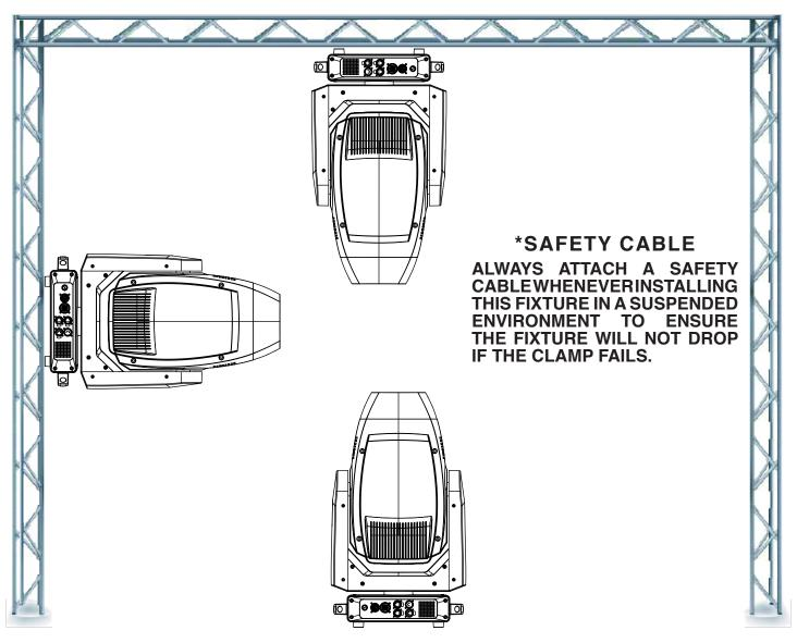
The Focus Spot 7Z is fully operational in three different mounting positions, hanging upside-down, mounted sideways on trussing, or set on a flat level surface. Always use and install a safety cable as a safety measure to prevent accidental damage and/or injury in the event the clamp fails. Never use the carrying handles for secondary attachment.
