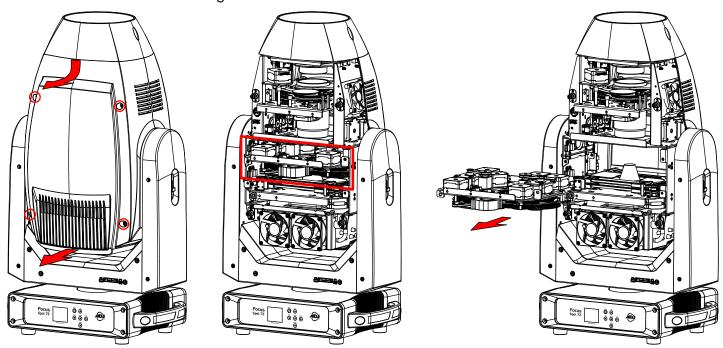
Locate the specific Rotating Gobo to replace. Carefully grip the Gobo using your thumb and index finger, gently lift it slightly, and then pull it out and away until it fully clears the Gobo Wheel.
