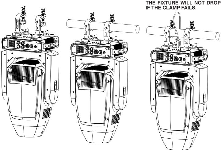
When installing the unit, the trussing or area of installation must be able to hold 10 times the weight without any deformation. When installing the unit must be secured with a secondary safety attachment, e.g. and appropriate safety cable. Never stand directly below the unit when mounting, removing, or servicing the unit.
