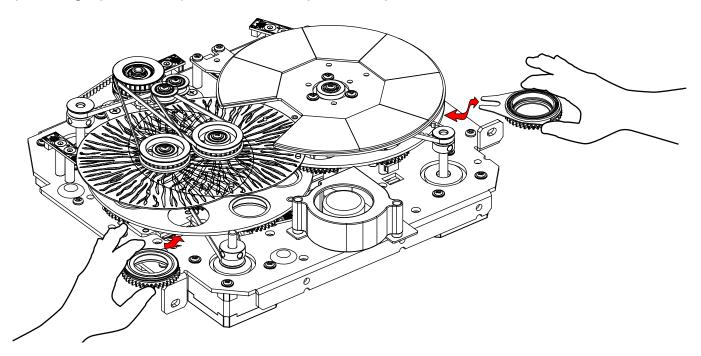
On the Gobo Holders, remove the retaining spring and carefully separate the GOBO from the GOBO Holder. Lastly, remove the flat washer attached to the removed GOBO and attach it to the desired replacement GOBO. Install the replacemet Rotating GOBO.
