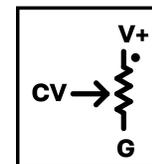
Do not use any other ground source. If multiple remote DC level controls are used for different channels, the same ground and V+ sources can be shared.
