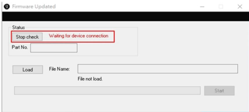
8. Please re-plug the USB cable and then please press the “Load” button to load the “CAP-1\_Main\_VX.X.bin” file.
