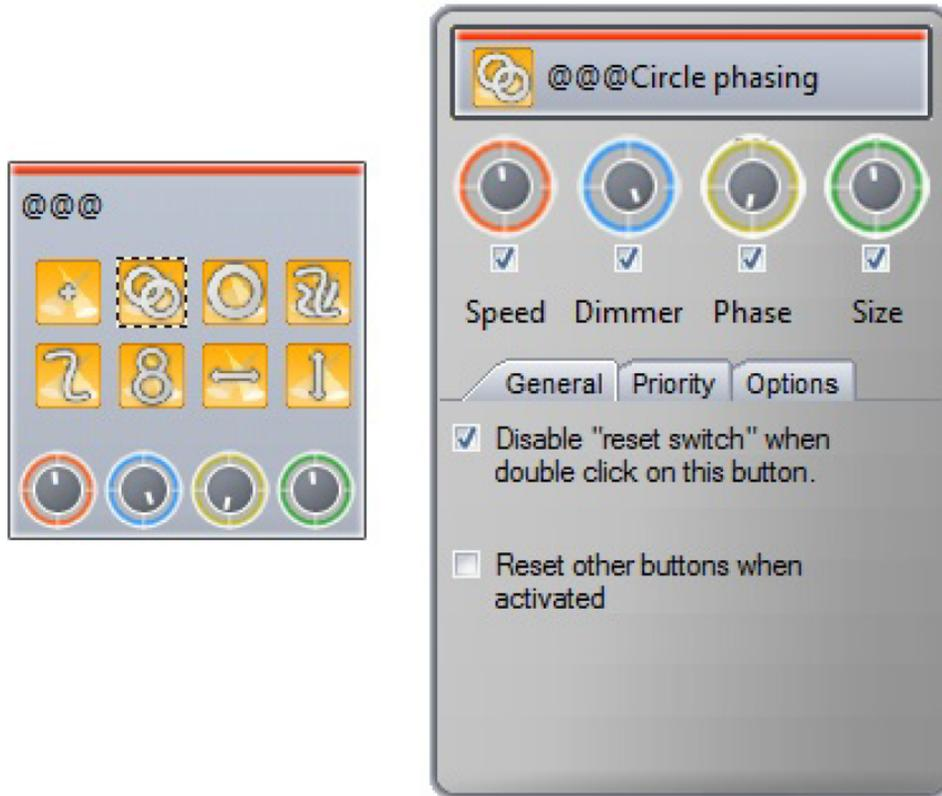
Speed, Dimmer, Phase, and Size dials can also be accessed under the button tab at the top of the fixture page. Page dimmer and speed dials can be accessed under the page tab, but be careful, if you turn the page dimmer to 0, you will never have any light output!
