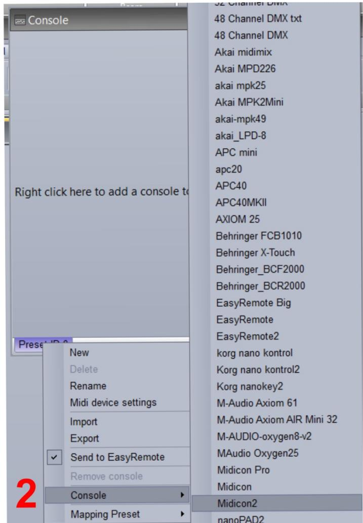
EasyRemote consoles are automatically mapped; however, with a MIDI or DMX console, you will need to set up the mapping. As with the EasyRemote consoles, many of the pre-built consoles are also mapped, so in some circumstances you will need to map each button/dial/fader on your controller to the console in the software.
