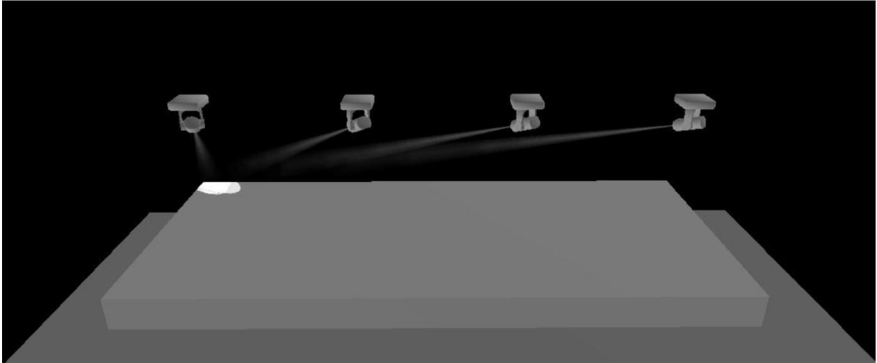
Click the '+' button to add a new calibration point, such as when moving the master and slave fixtures to the center top of the stage. A quick way to do this is to select all fixtures and hold ctrl whilst moving the point on the X/Y grid, this way all fixtures stay close and you can perfect the calibration using the arrow keys.
