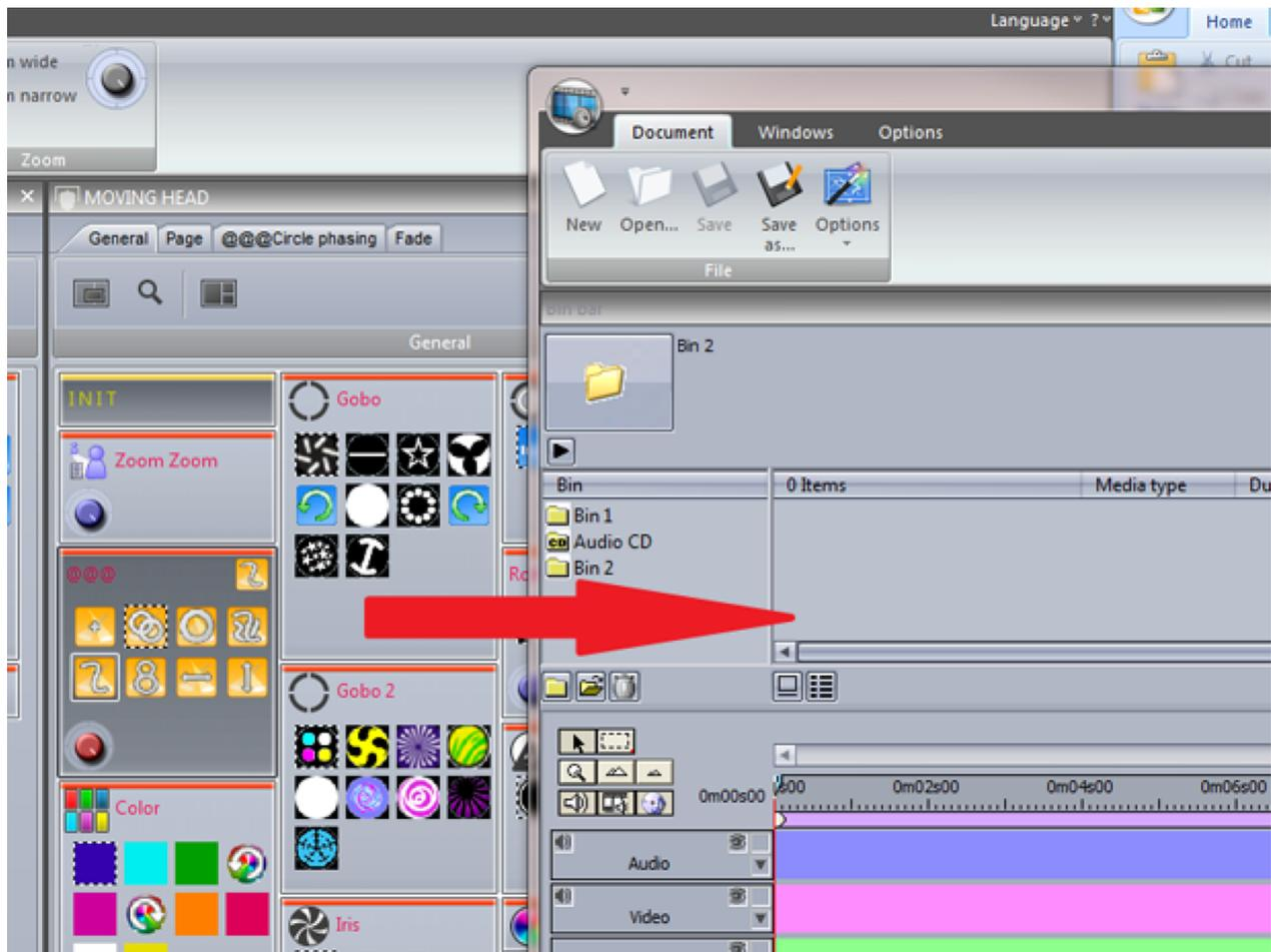
A new track is automatically set up for the page. The scene can now be dragged onto the new track. Note how the track is split into two sections, the top section for SCENES and CYCLES, and the bottom section is for SWITCHES. If you need more than one Switch activated at a time, click here (1) to create a new Switch timeline.
