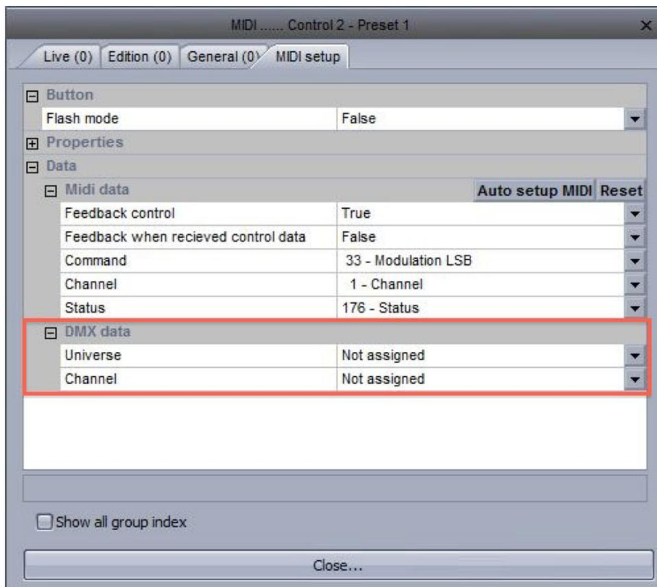
Once the DMX controller is mapped to the Console, you can map the controllers, faders, dials, and buttons to almost any software feature; see the Console topic for more information.
