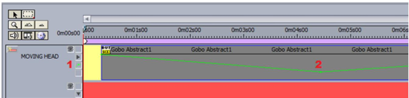
Marker points can be added to the timeline and used to stop playback. If 'Jump in playback mode' is selected, playback will continue when the marker is reached.
