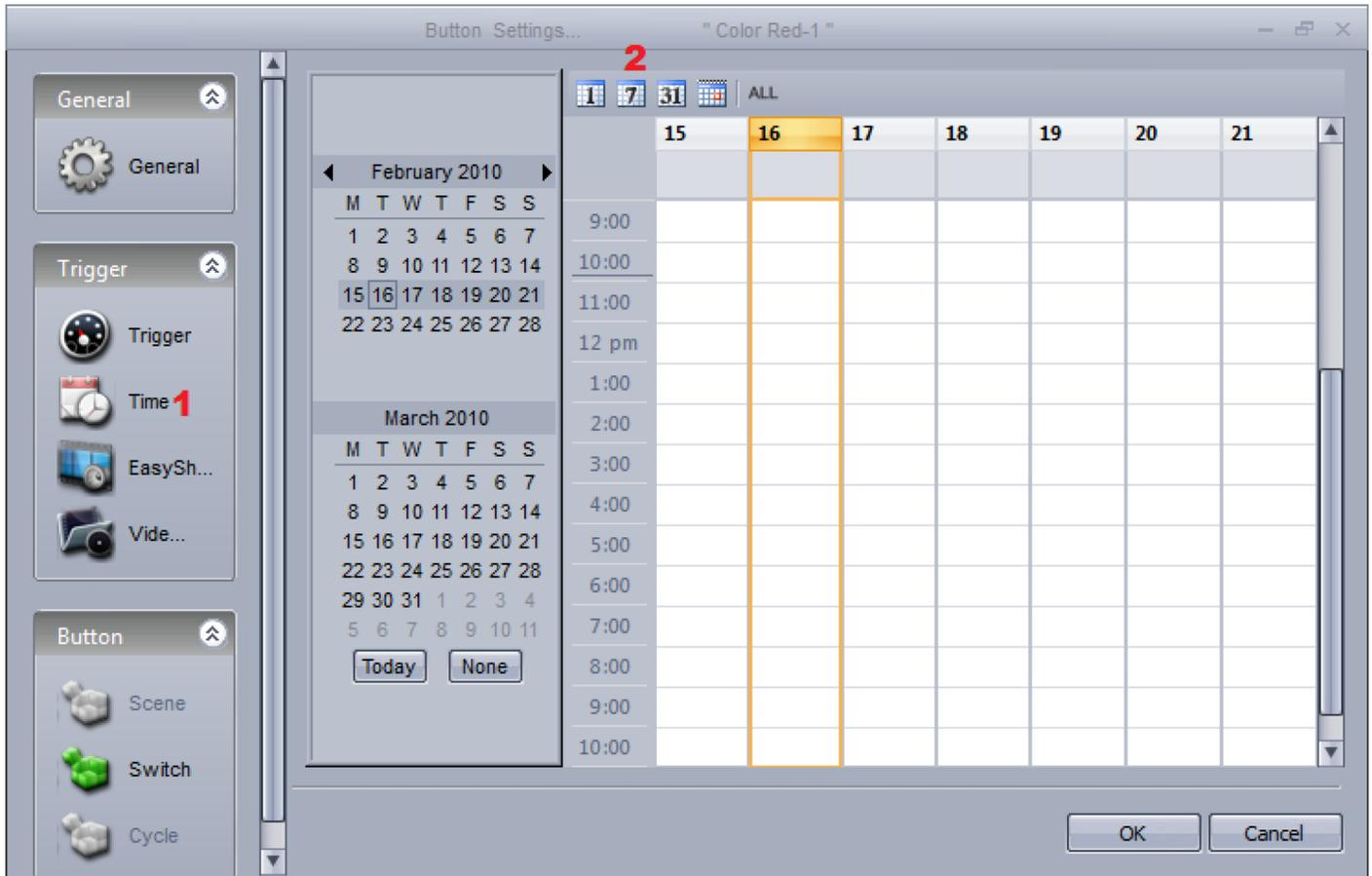
Scenes can be triggered at sunrise and sunset. A custom location can be assigned by clicking here (1) and the time of sunrise and sunset will be automatically calculated. A trigger time relative to the sunrise or sunset time can be assigned here (2). For example, a scene could be deactivated 4 hours after sunrise.
