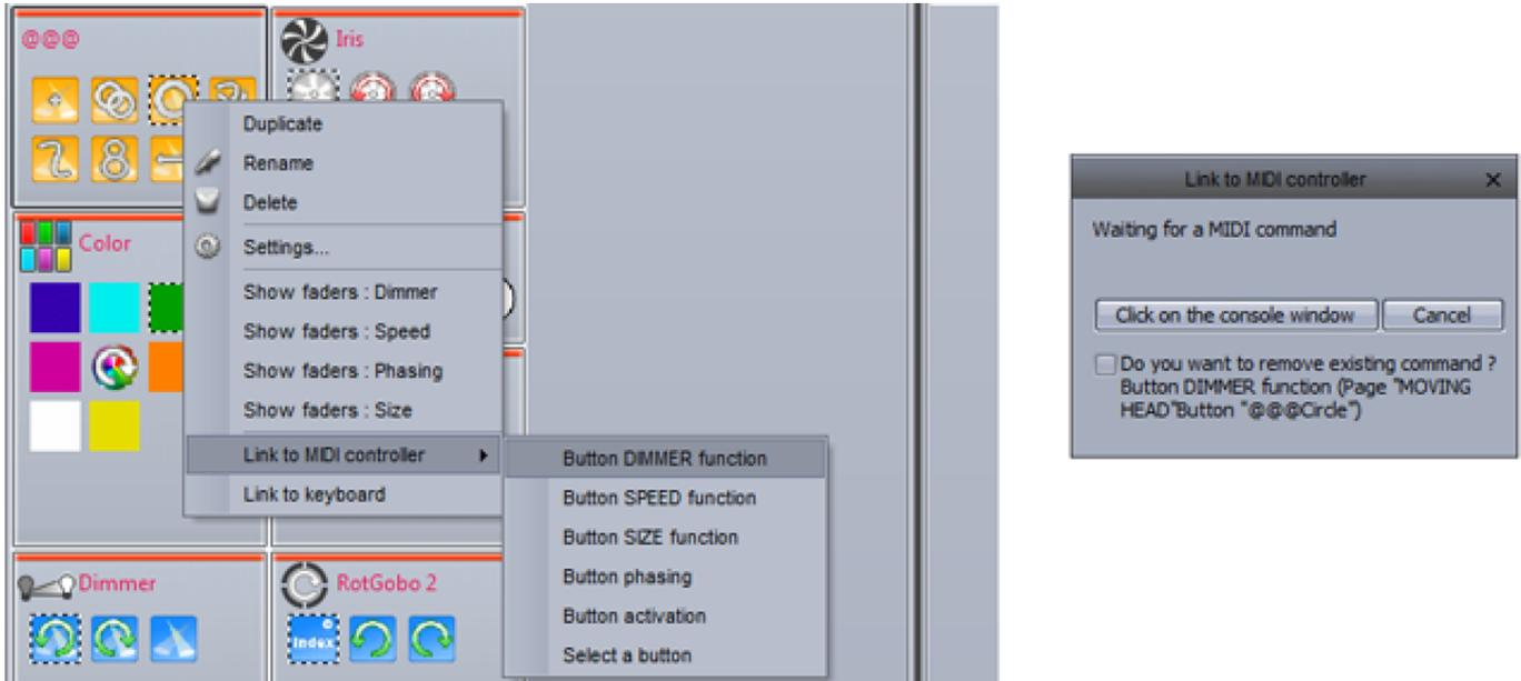
One command on the controller can be used to activate a variety of different commands within the software. For example, you could assign a dial to automatically control the speed of several movement buttons. Commands can be edited by right-clicking on the relevant button on the console. Here we can set a minimum and maximum value to trigger the command. In the example below, when the input value reaches 47, the sequence will be at maximum speed.
