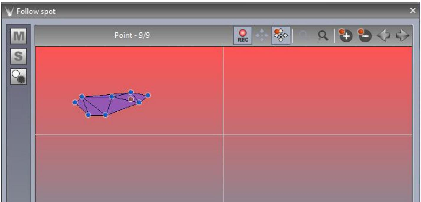
Once the editor has been closed and saved, all slave fixtures will follow the master fixture as long as the switch is activated. The switch works in 'Always take priority' mode to override any pan/tilt values on slave fixtures.
