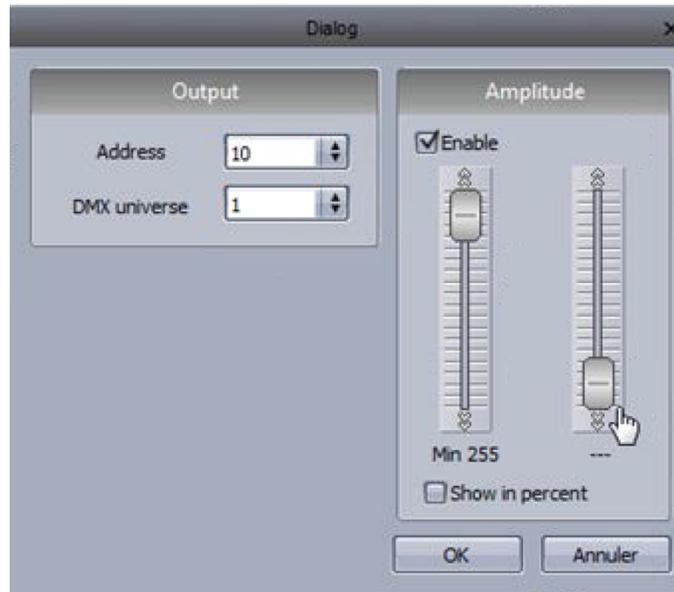
It is possible to limit the highest pan and tilt value of a fixture. This is useful if you have a fixture in the corner of a room and you don't want the fixture to point at the wall. It can also be used to calibrate a fixture's moving sequences if not programmed with palettes:
