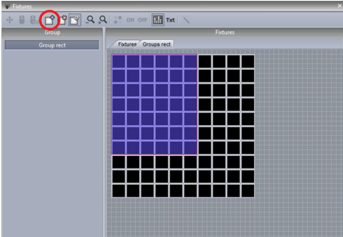
To apply an effect onto a rect, drag the rect onto the timeline to create a new track. You can drag your effects onto the timeline in the usual way.
