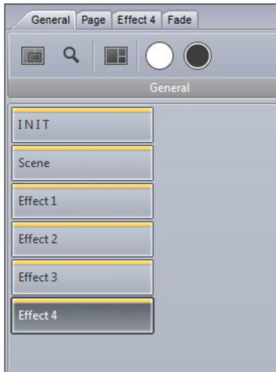
Button compression types can be modified within the page settings. Create a new compression here and enter the compression prefix, in our case this is 'Effect.'
