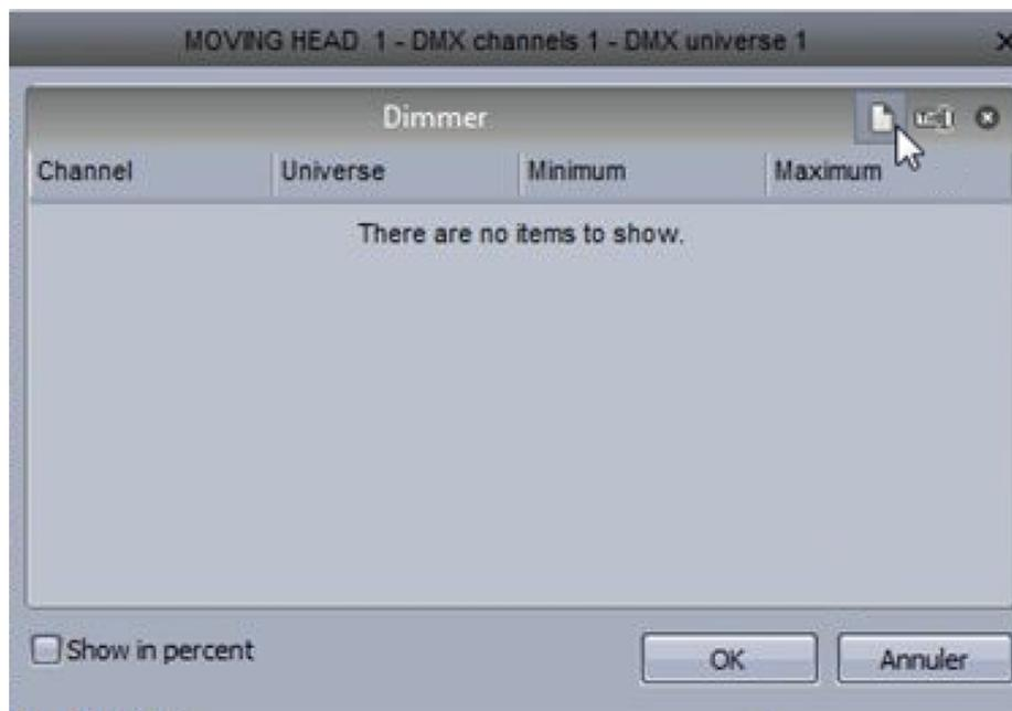
The output channel and universe can be set on the left, and the minimum and maximum amplitude can be set to scale channel values down. Setting the minimum to 255 and the maximum to 0 will invert the channel. This can be useful when using unusual fixtures whereby the dimmer is at 100% when the channel is at 0.
