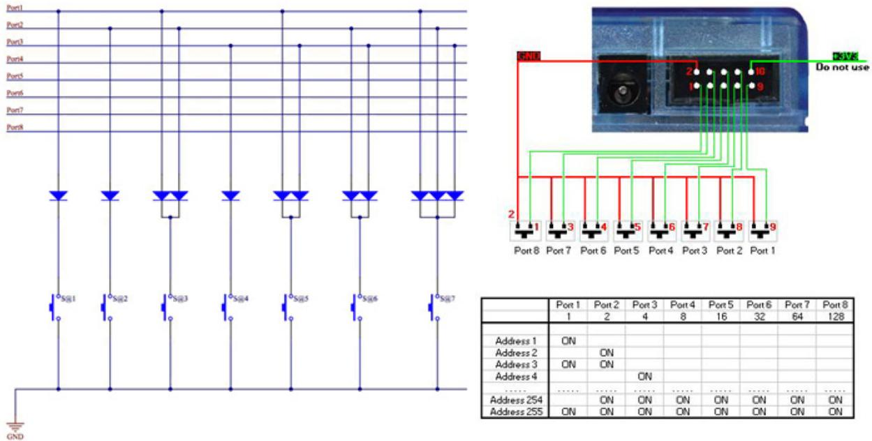
Once the port connections have been set up, they can be assigned to trigger a scene within the scene settings 'Trigger' tab. If you are addressing the ports in binary, be sure to select 'Address 8' instead of 'Port 8.'
