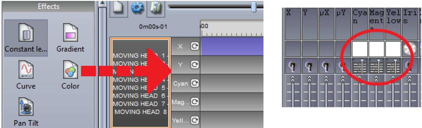
If the constant level effect is dragged onto a pan/tilt channel of a moving fixture, the position can be modified by dragging on the X/Y grid, or by choosing a palette if one has been created.
