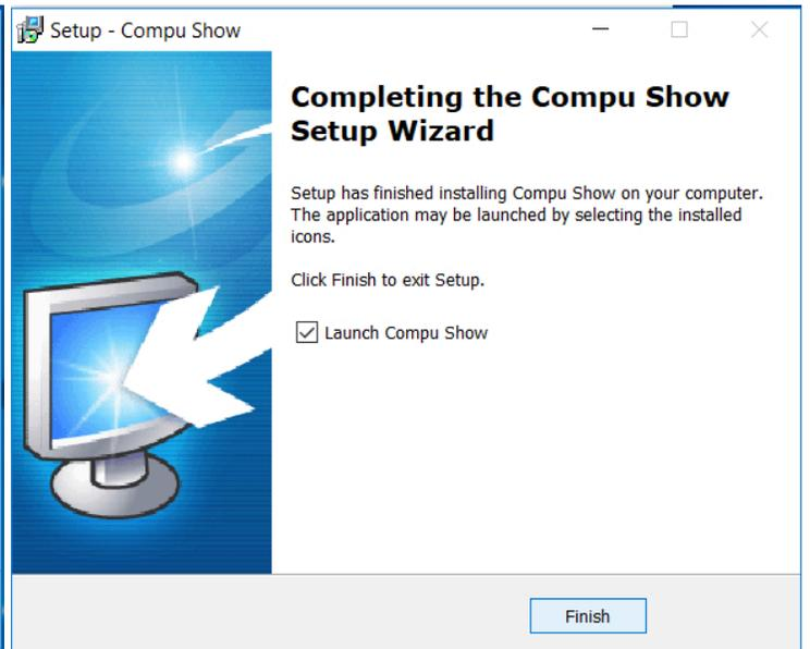
The DMX interface USB drivers will be installed during the software installation. When the Windows driver installation dialogue appears, click next. If a dialogue appears to say that the drivers are not digitally signed, select 'Continue Anyway.'
