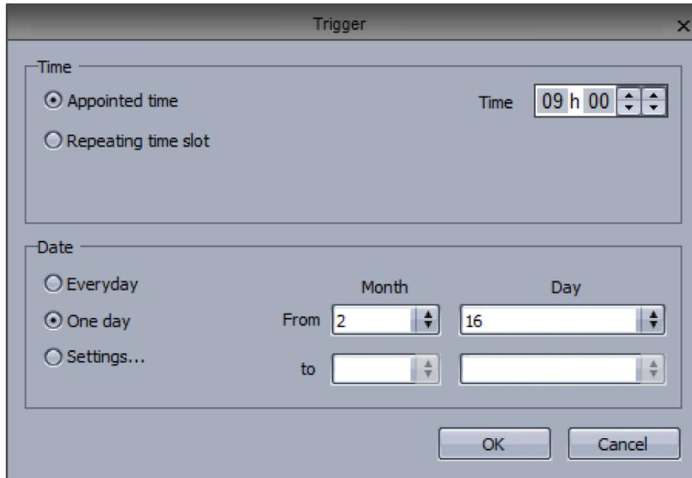
Note that the time triggers created within the button settings are not applied in stand-alone mode. Once the stand-alone scenes have been created and assigned, the memory can be written here (1).
