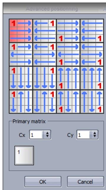
Imagine that you have a single fixture composed of 4 RGB devices, all of them positioned on a 2x2 matrix (12 DMX addresses). In some cases, you may want to treat these 4 fixtures as 1 fixture. In this case, you can set up a primary matrix. Select the primary matrix dimensions and drag the fixture positions if necessary.
