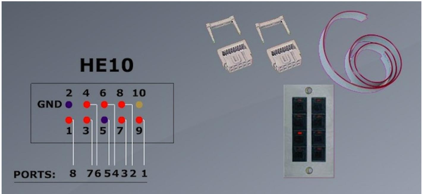
You can connect up to 255 buttons by combining the 8 ports into binary. For example, if ports 1, 2, and 3 are connected to the ground pin, this will trigger address 7.
