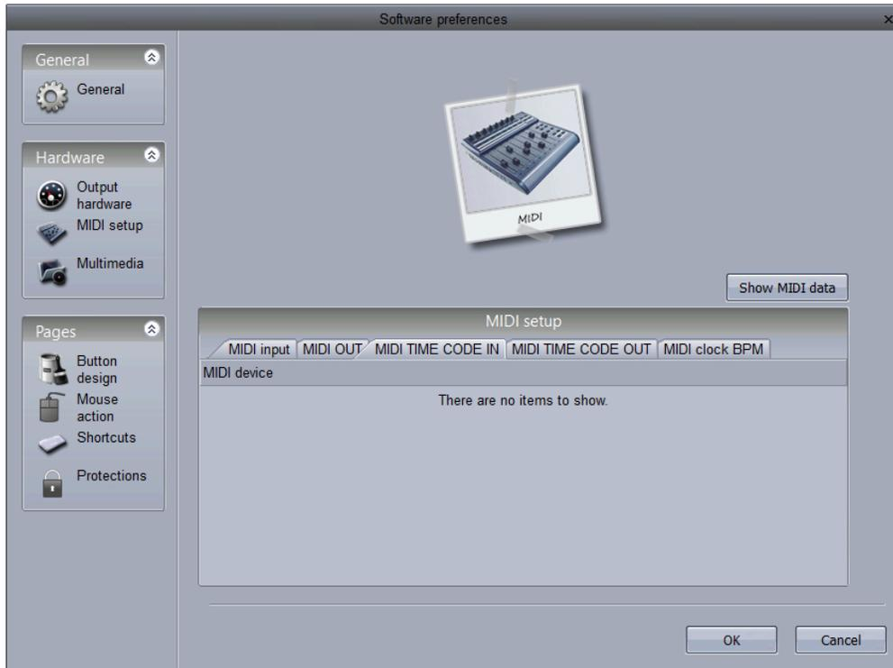
Once you have your MIDI Time Code device connected, select the IN button to begin receiving the Time Code signal. To send Time Code to another device whilst the Cycle is playing, select the OUT button.
