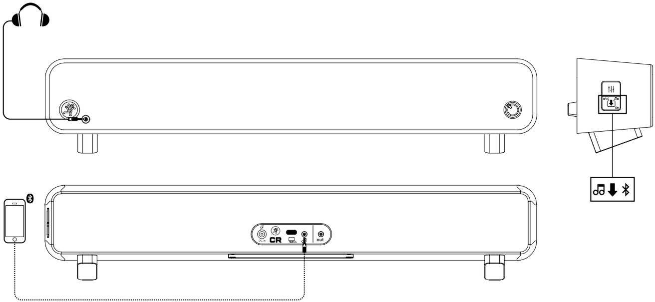
The illustration above shows another typical use for CR StealthBar. This would be a prime example of utilizing it to play music. Make sure the CR StealthBar is positioned for your setup, including the angle; see 'Adjustable Feet' on page 9 for more information.
