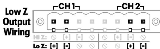
Speaker connections are configured for either high impedance output (Hi-Z), or low impedance output (Lo-Z) using the DIP switches as shown in [section 5.2a](#).
