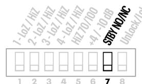
when the standby pin is pulled high or left unconnected.
