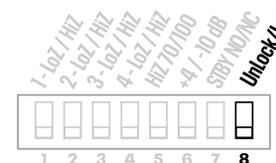
*Note: Remote DC level (VC) inputs continue to work normally even when front panel controls are locked.*
