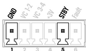
When the amplifier is put into standby mode using the STBY contact closure, automatic sleep mode wake-on-audio is disabled, and the front panel power switch is also disabled.
