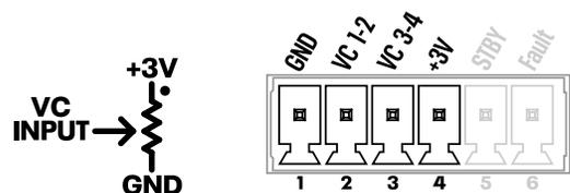
On the two-channel model (not shown), each VC input controls its own channel. On four channel models (shown), each VC input controls a channel pair. The maximum volume when using remote DC voltage control is set by the front panel level knobs. See the diagram above for proper wiring.
