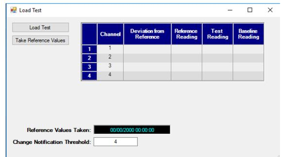
Note that certain level controls for high impedance speakers (such as those manufactured by Atlas and Lowell) adjust volume by changing the load impedance. In this case, changing the volume will result in a variance reported by the application.
