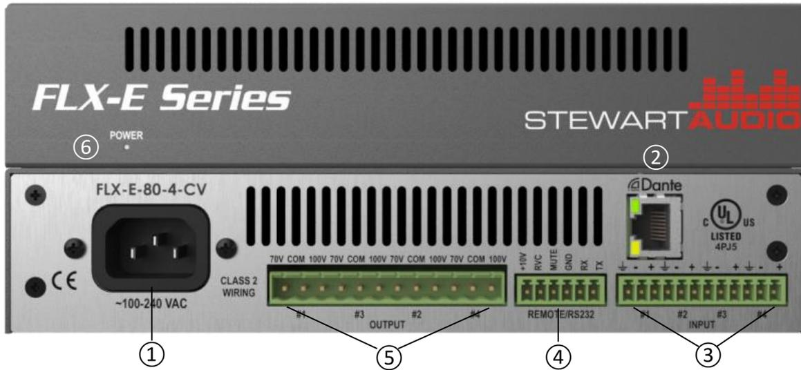
1. **AC line input** – Connect the included IEC power cable.
