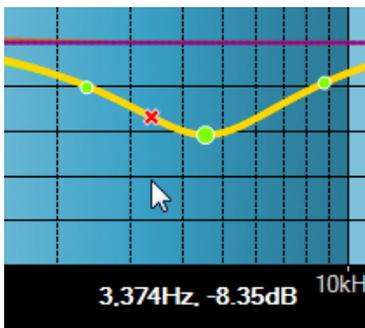
To check values on the cascaded filter frequency response, click anywhere on the graph (other than on drag markers) and red crosshairs will appear on the cascaded filter moving the mouse horizontally will drag the crosshairs along frequency axis displaying the gain level at the corresponding frequency.
