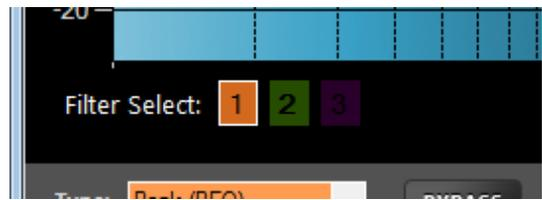
When a filter is selected, drag markers appear for that filter to allow configuration of center frequency, gain, and bandwidth (Q).
