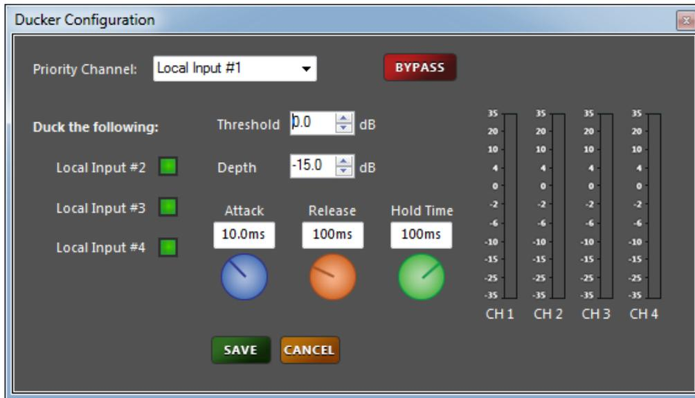
**Priority Channel** is a dropdown to select the channel which is given priority and which will activate the ducking (attenuation) of other selected channels, when the signal level of the priority channel reaches the set threshold. The dropdown menu will display the name set in the channel's input configuration.
