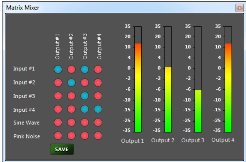
**Signal Generators** are included on the input list in order to provide signals for testing purposes. The generators include a sine wave and pink noise generated at 0dB. The frequency of the sine wave is fixed at 1kHz and is not adjustable.
