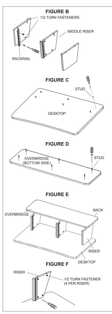
4a) If rackbays are needed, attach the rackrail to the risers as shown using flat head screws.
