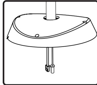
4. Run RJ45 signal wire and at least one safety cable through conduit.
