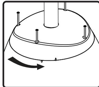
8. Line speaker up with cover plate and rotate to lock in to place. Alignment marks will meet when secured.
