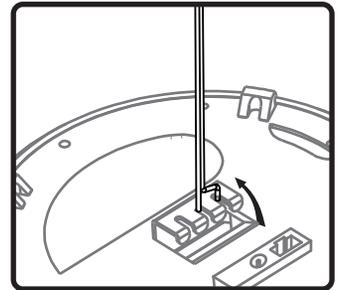
7b. Once aligned with central cable slot, pull cable up into slot to secure. Repeat steps 7a and 7b with secondary safety cable into one of the side slots.
