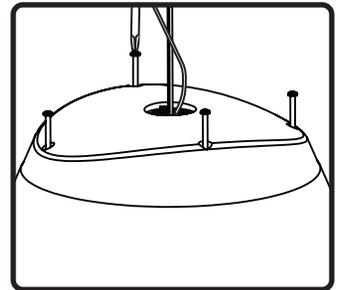
11. Tighten all four (4) screws to lock cover plate in place.
