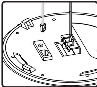
9. Plug RJ45 connector into speaker. If local power\* is required at speaker (non-POE installation), connect appropriate DC power supply to barrel connector on speaker input panel.
