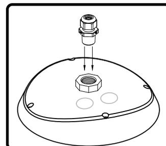
2. Thread the 3/8" NPT wire gland into the 3/4" to 3/8" NPT adapter. Make sure to tighten securely to ensure a water tight fit.
