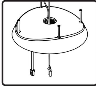
6. Slide cover plate over hanging and safety cables and run RJ45 signal wire through center hole.
