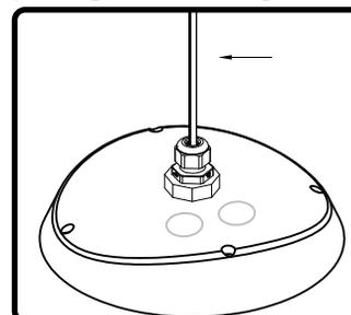
3. Thread the speaker security cable and ethernet cable, prior to terminating the RJ45 connector, through the 3/8" NPT wire gland and attach to the back of the speaker as noted in previous instructions.
