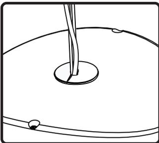
12. Install rubber weather plug by sliding slit over the wire, then pressing snugly into hole in cover plate.
