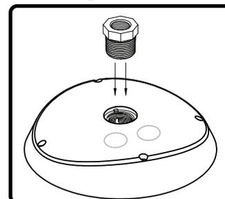
1. Thread the 3/4" to 3/8" NPT adapter into the the top plate of the speaker in the hole provided. Make sure to tighten securely to ensure a water tight fit.
