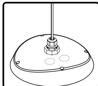
4. Tighten the top of 3/8" NPT wire gland such that the rubber grommet is tight around the cable. *This may require a wrench.*
