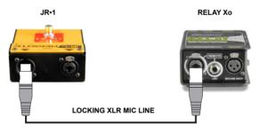
Another advantage is that XLR cables can be dasiy-chained together to make a longer cable. This means you won't have to depend on a specific custom built cable to connect your remote device.
