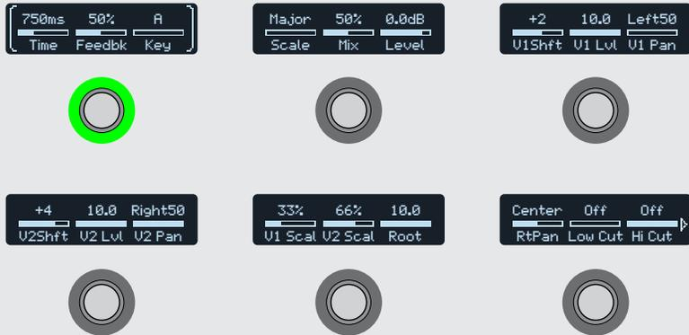
Touch the desired footswitch to select its parameters and then turn knobs 1-3 to adjust them. If a block has more than 18 parameters, press  $\triangleright$  to access more parameters. When finished, touch a switch for one second (or press  $\text{HOME}$ ) to exit.
