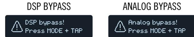
**NOTE:** There are two types of All Bypass for the HX Effects device: Analog bypass (sometimes called "true bypass"), where mechanically switching relays route your signal directly from the inputs to the outputs with no processing or A/D/A conversion, and DSP bypass, where any delay echoes and reverb tails decay naturally. By default, the HX Effects hardware is set for Analog bypass, but this behavior can be set from ["Global Settings > Preferences"](#)
