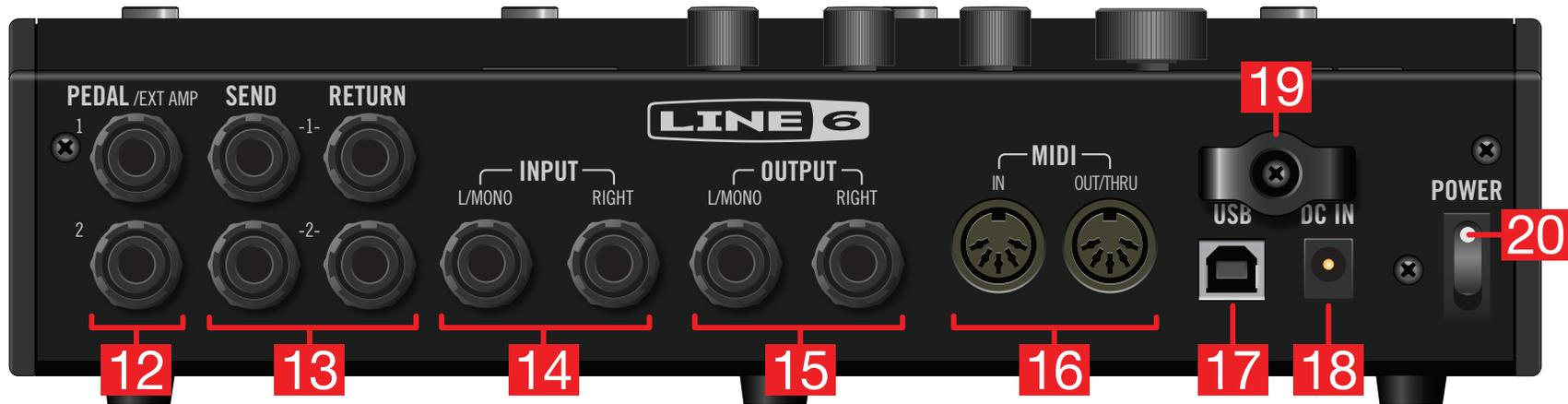
**12. PEDAL/EXT AMP 1-2** Two expression pedals can be connected to the HX Effects device and assigned to adjust a wide variety of parameters. By default, EXP 1 is automatically assigned to control and bypass Wah/Pitch Wham type blocks, and EXP 2 is automatically assigned to control Volume blocks, making them ready for use with your connected expression pedal(s). See ["Assigning a Controller"](#)
