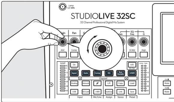
You can now control the preamp level and phantom power for your NSB stage box from the Fat Channel on your console, in the same way that you control the local inputs.
