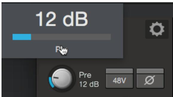
You can now control the preamp level and phantom power for your NSB stage box from the Fat Channel in UC Surface, in the same way that you control the local inputs.
