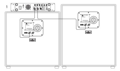
A speaker cable with Speakon ends connects from one Speaker Output of the amplifier to the Speaker Input of an Ampeg Pro Neo PN-115HLF cabinet. Additionally, an Ampeg Pro Neo PN-410HLF cabinet is connected from the remaining Speaker Output of the amplifier to the cabinet's Speaker Input using a speaker cable with Speakon ends.
