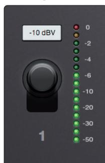
When a 1/4-inch TRS cable is connected to the inputs of your Quantum-series interface, you will be provided with an input sensitivity toggle switch. By default, the input sensitivity is set to +4 dBu. Most professional line-level devices output at this level. Consumer line level is usually -10 dBV. For these lower output devices, switch the input sensitivity to -10 dBV to match your device.
