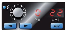
**Preamp controls.** These controls allow you to adjust the gain and enable phantom power for every onboard microphone and instrument preamp.
