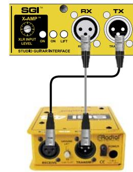
Fig.36 - Balanced XLR connections between the JX44 and SGI-44.
