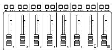
Adjust output of each channel.
