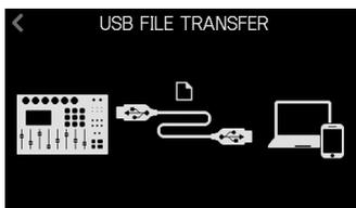
3. Use a USB cable to connect the **P8** with a computer, smartphone or tablet (→ page 11).
