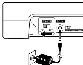
1. Plug the specified adapter (AD-14) into an outlet.
