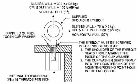
**DIAGRAM: Cross-section of Mounting Rigging Point**
