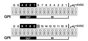
The DME7 has 16 input terminals and 8 output terminals.
