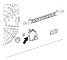
2. Insert the other end of the hook into the upper end of the security slot.
