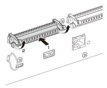
2. To remove a Euroblock plug, lower the left and right locks, and then pull out the plug.
