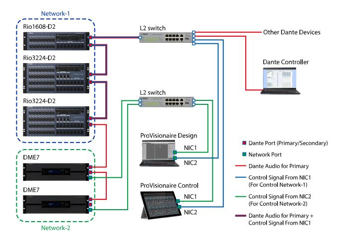
The appropriate latency setting for signals sent and received over a Dante audio network differs depending on the connection method and scale. The following is an explanation of how to select the [Latency] setting based on the connections between Dante-compatible devices and the DME7.
