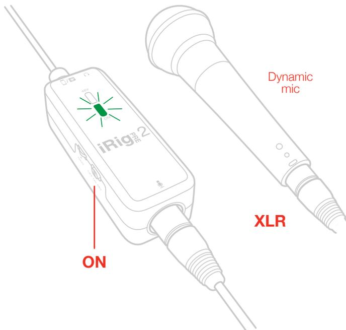
5. If you are using a microphone that needs phantom power (like most condenser microphone), slide the power switch to the upper position (marked +48V) to turn phantom power ON. The red LED will light.
