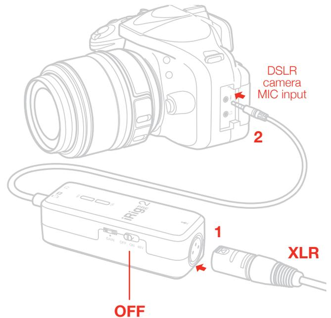
4. Turn the iRig Pre 2 ON by sliding the power switch to the ON position. The green LED will light.
