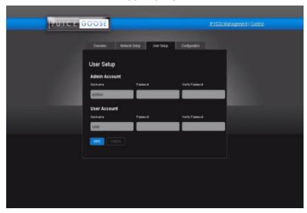
The user setup tab is where you configure the Admin and User account passwords. You can change the username and password on both accounts by typing in the changes in the corresponding fields. There is a second password field for both accounts that verifies you typed the password in correctly. If you did not, an error message will be displayed when trying to save the changes.
