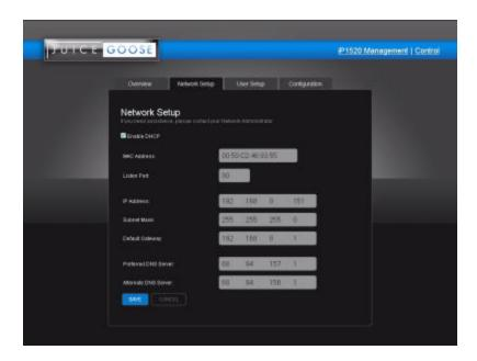
In the above screen capture you can see the network setup tab accessible when logged in as Admin.
