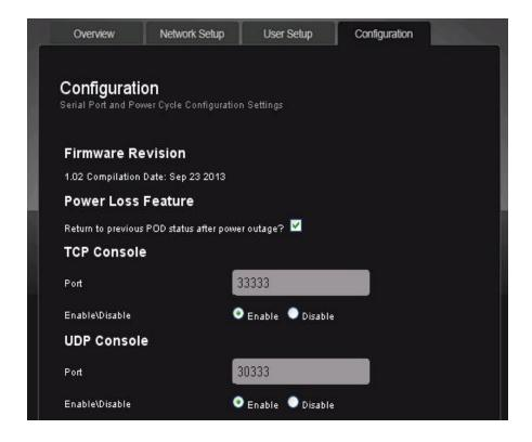
To connect to IP1520 over TCP, simply start your TCP client program ( such as Hercules or PuTTY) and specify the IP address of the iP1520 and the TCP port. Start the connection ( many programs have a Connect button to start the connection ) and type iP1520 console commands such as Help. You should see the reply to the command on the TCP client terminal window. See page 13 and 14 of this manual for a full list of the console commands available.
