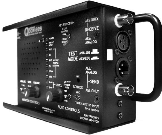
The Whirlwind Qbox-aes is a multipurpose testing device for troubleshooting digital AES-3, S/PDIF and analog audio signals. It is composed of two sections; a Send section and a Receive/Monitor section. A Test Mode switch selects Analog or AES testing operation. Audio is decoded and output through the built-in speaker or the 3.5mm jack. Test signals can be generated from multiple sources. In Line monitoring of an AES data stream is also possible with no alteration of the signal passing through.
