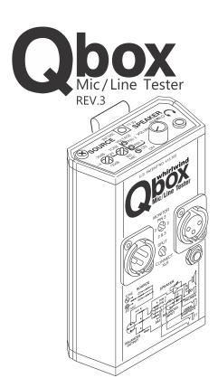
The Qbox is a multipurpose testing device used for checking audio lines. The Qbox can send or receive audio signals at either mic or line levels, as well as detecting the presence of phantom or intercom voltage on the line.
