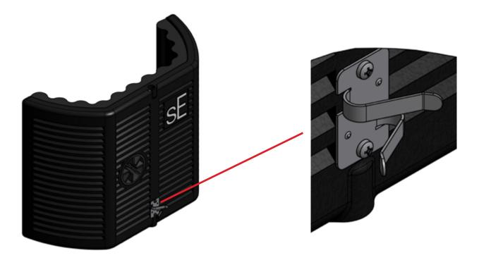
Using a Phillips-head screwdriver, attach the bracket to the filter using the two small included screws, through the two pre-drilled holes in the back of the filter (as shown above). You can then fit one or two mic cables under the clips, gently folding the clips over the cables to keep them in position.
