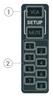
The VCA setup is enabled by pressing the VCA key, it then uses the mute masters in conjunction with input channel SELect keys to configure input channels as slaves to a VCA master.
