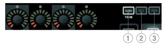
The Global Mode encoders offer control of a key parameter across all channels or buses currently active on the surface:
