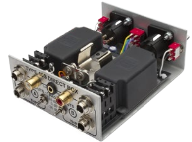
Inside of the Type 10S DI: the circuit board is protected by a solid block of epoxy.
